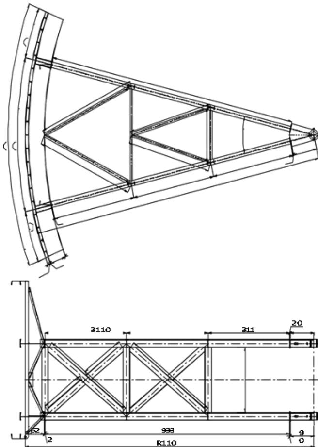
Fig 2: Layout of radial gate
